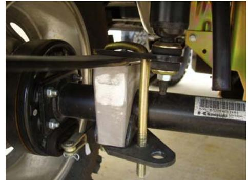
**\*\* These spindles are pre-drilled to accept Jake's hydraulic front brake kit. \*\***
